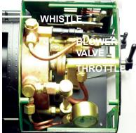
It will take approximately 7 minutes to raise pressure. Once the gauge reaches 20 lbs, you can shut off and remove suction fan from the stack and then turn on the engines internal blower. At this point steam will rise rapidly!
