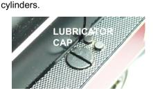
ensures the cylinders and valves are properly lubricated inside. As the steam passes through it, a small
